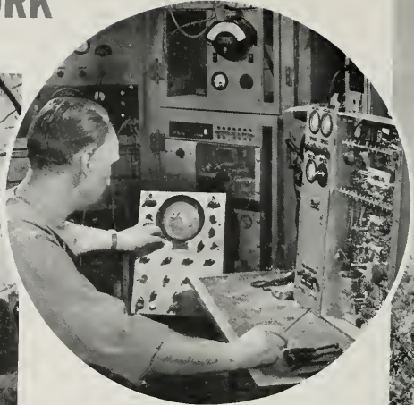
THE OSCILLOGRAPH PROVIDES A "PICTURE" OF THE PERFORMANCE OF RECEIVERS.
